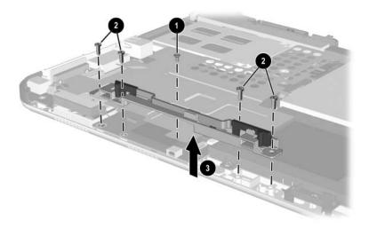
Removing the Keyboard Release Assembly
